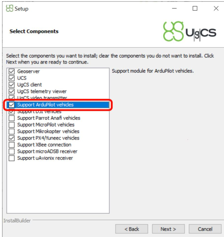
Figure 4.18 – UgCS installation Support for ArduPilot vehicles
