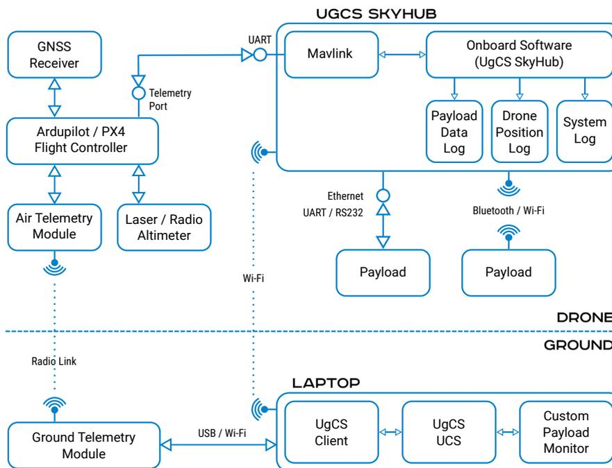
Figure 1.2 – Pixhawk autopilot based drone interaction diagram
