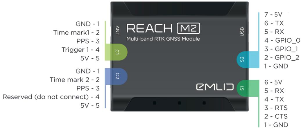
Figure 5.2 – Emlid Reach M2 Port Pinouts
