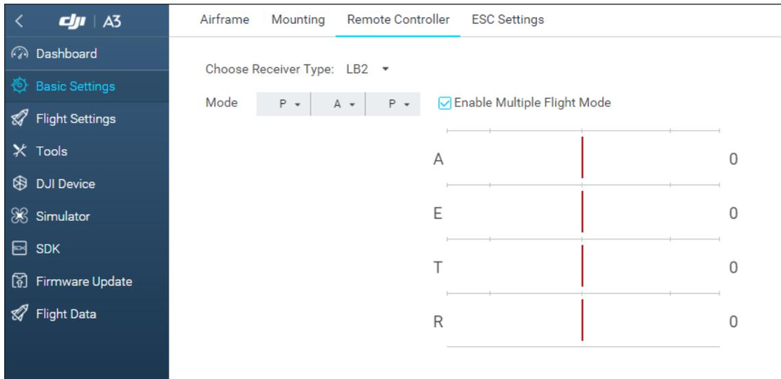
Figure 4.11 – Enable API control in DJI Assistant 2
