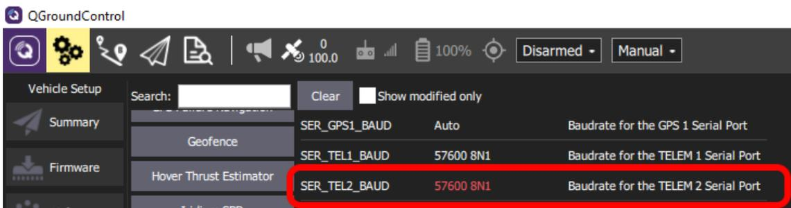
Figure 4.27 – UgCS SkyHub PX4 TELEM2 port baudrate configuration
