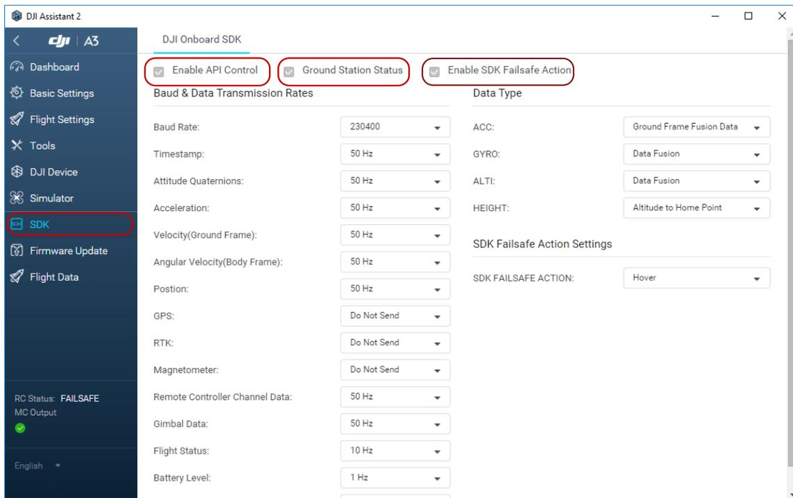
Figure 4.10 – Enable API control in DJI Assistant 2
