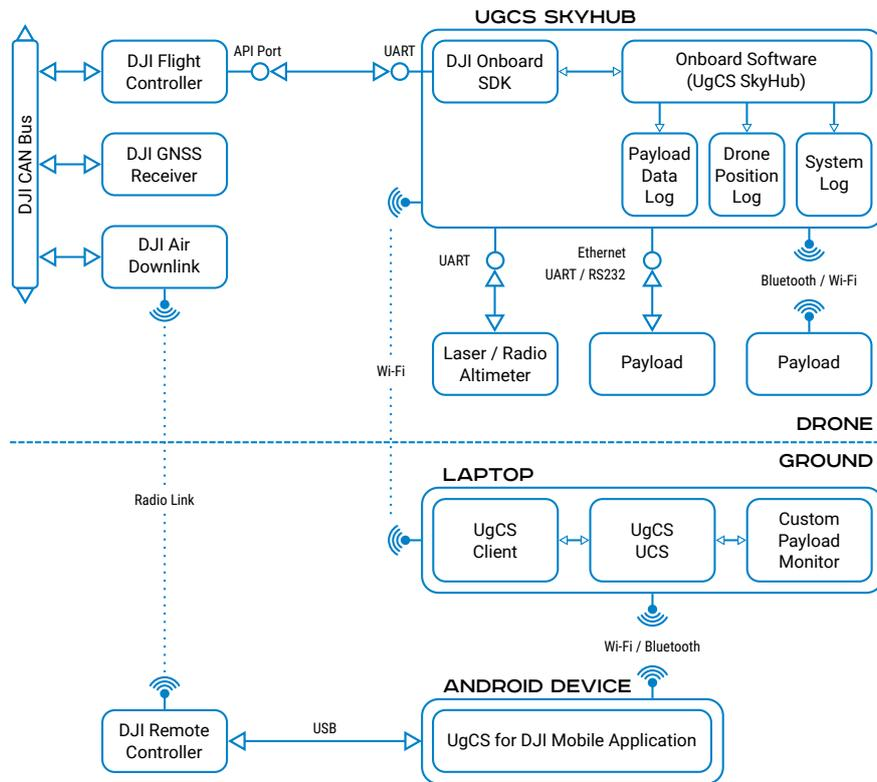
Figure 1.1 – DJI SDK drone interaction diagram
