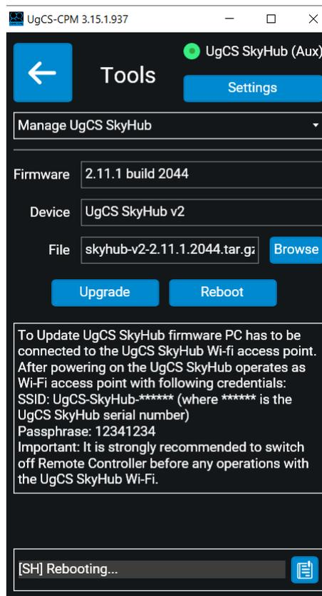
Figure 6.5 – UgCS-CPM. Manage UgCS SkyHub window
